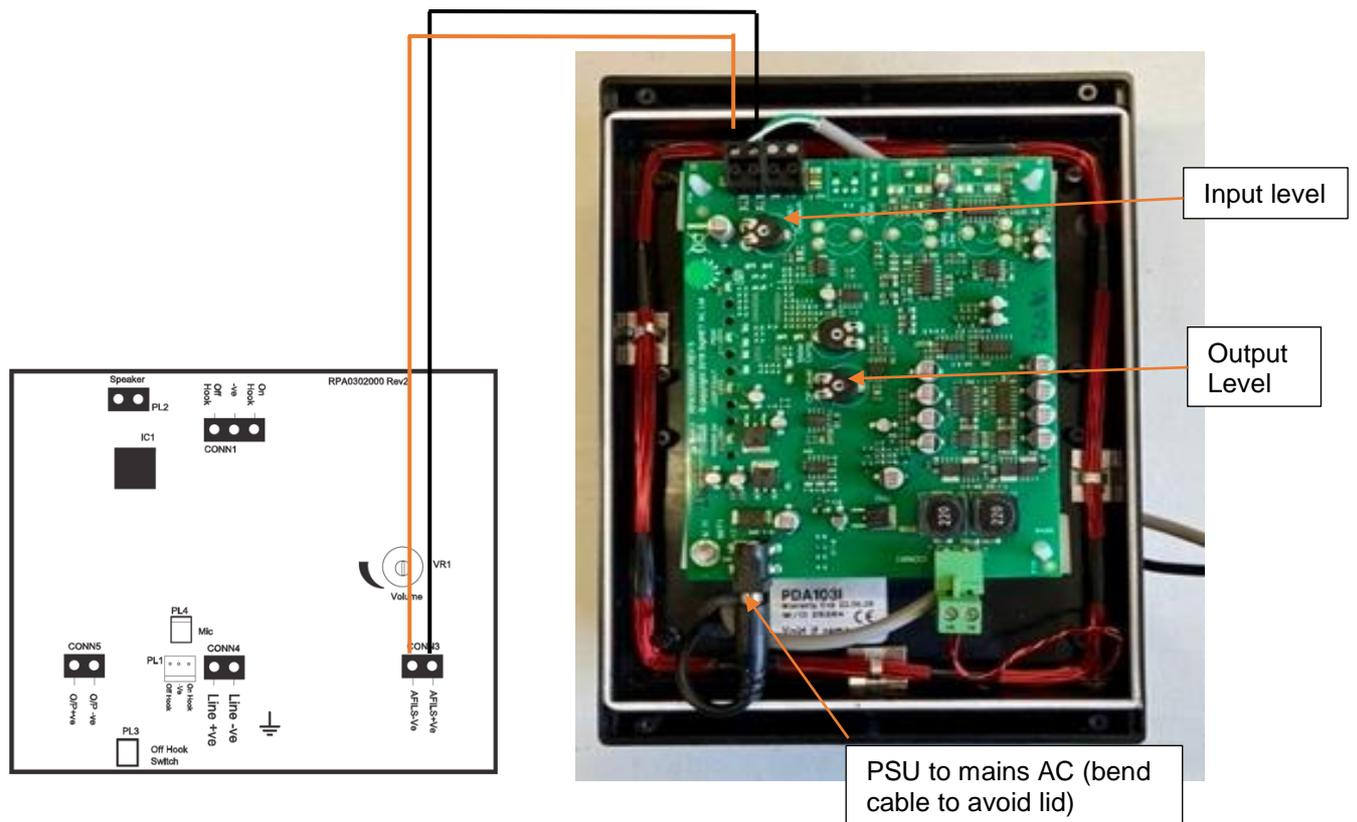
In the event of no plug socket being available, the Mains PSU can be replaced with a 14 to 20V DC 0.9A mains power supply.
