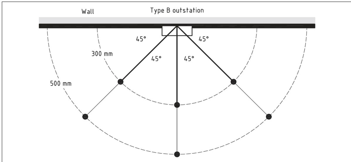
Note: Where an audio frequency induction loop system is provided at an outstation, it should be installed and maintained according to the recommendations of BS 7594. The performance of the audio frequency induction loop system should meet the requirements of BS EN 60118-4 at the six locations shown in Diagram 2, namely 400 mA/m
